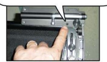
Then slide the locking bolt down, tighten the bottom screws and replace the top screws into the two top holes.
