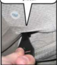
Attach the top and bottom strap and pull to tighten. The straps should be snug so there is no slack but do not need to be very tight.
