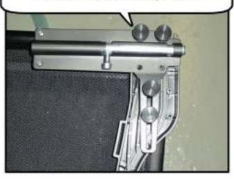
Your wind deflector will fit in the trunk when not is use. Start by folding it up. Then place the locking bolt side in first.
