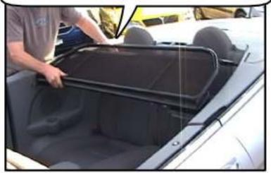
The rear bracket will enter into the holes on each side of the rear trim panel.
