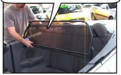
Unfold the bottom panel out towards the rear seat. The wind deflector will bend in the middle and lay flat.
