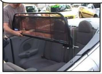
Slide the plastic locking bolt into the hole in the trim panel on the opposite side from where you are standing.
