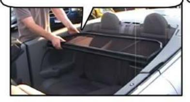
Now just lift up on the rear of the front panel and the rear brackets will slide out. Unlock the locking bolt on the side closest to you and lift the wind deflector out.
