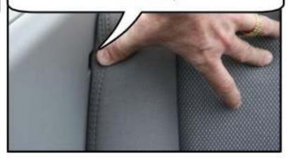
Place one hand on the bottom of the front panel and one hand on the bottom of the back panel.
