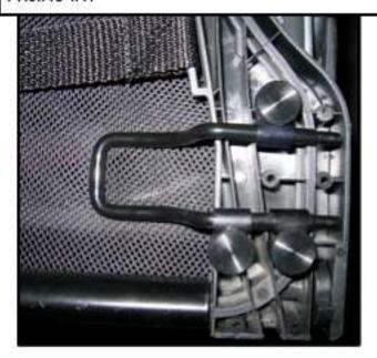
STEP 1 CONT LOOSEN ALL THREE SCREWS, TURN THE BRACKET SO IT FACES OUT AND THEN TIGHTEN. REPEAT TO THE OTHER SIDE
