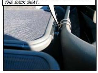
STEP 3: THE TWO SCREWS THAT NEED TO BE REPLACED ARE ON THE TRIM PANEL BESIDE THE TOP OF THE BACK SEAT.
