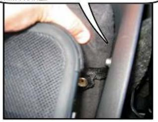
STEP 4: NEXT ATTACH THE FRONT HOOK STRAP TO THE BOTTOM SIDE OF THE TRIM PANEL. THESE STRAPS ATTACH TO THE FRONT BRACKET OF WIND DEFLECTOR
