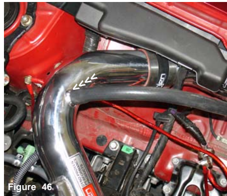
Figure 43 One end of the 17mm hose is inserted into the box spout until it is firmly in place.
