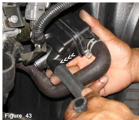
Figure 43 One end of the 17mm hose is inserted into the box spout until it is firmly in place.
