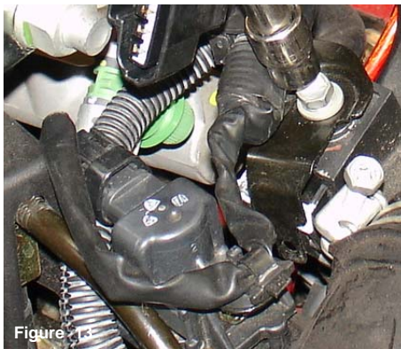
Figure 10 Loosen and remove the two screws located on the mass air flow sensor housing.
