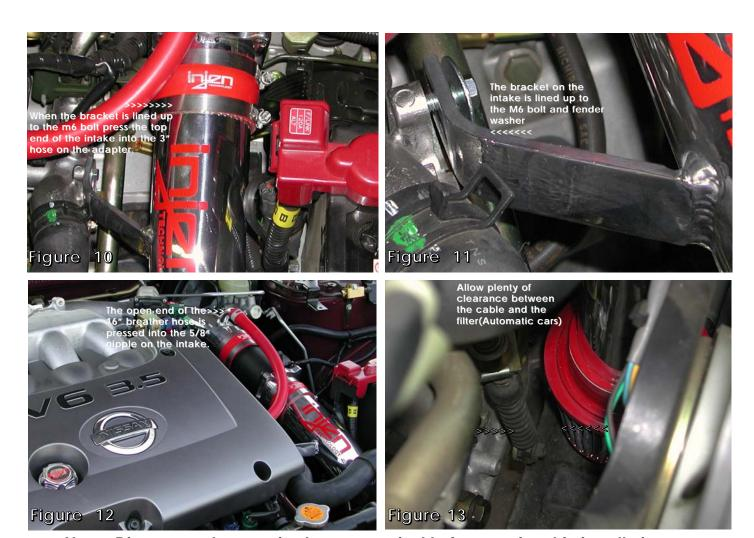
Note: Disconnect the negative battery terminal before starting this installation.
