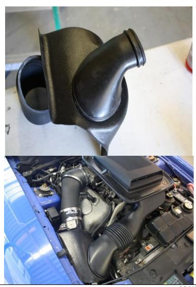
Go back and make any adjustments to the tube and tighten the clamps (**ONLY FINGER TIGHT**). Installation is complete.
