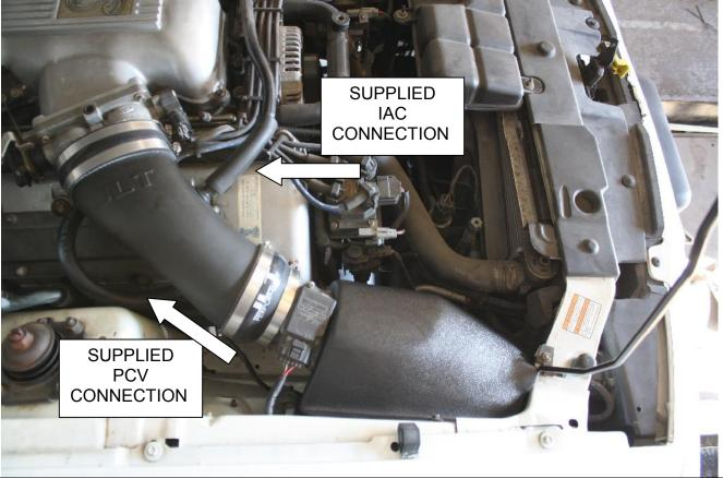
Go back and make any adjustments to the tube and tighten the clamps (ONLY FINGER TIGHT). Installation is complete.
