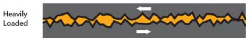
Boundary Lubrication - Performance Completely Dependent On Boundary Film Additive film wears instead of metal surfaces
