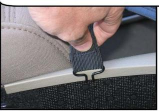
**Step 2 Cont:** Pull the strap snug and then fold the strap so the velcro secures it in place.
