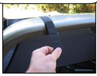
**Step 3:** Now attach the wind deflector to the back seat. Using the snap and the black book that attaches to the side of the tirm panel.
