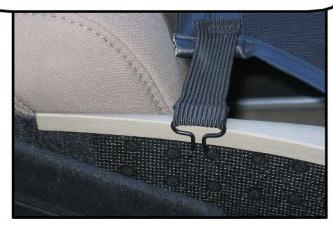
**Step 4:** Push the snap into place (this can take a bit of force) And repeat on the other side.
