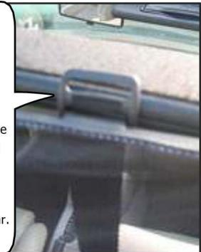
**Step 2:** The strap will wrap around the roll bar then go through the plastic slider.
