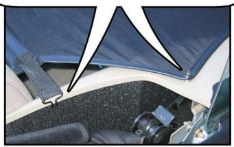
**Step 3 Cont:** Repeat on the other side. The elastic and hook will hold the wind deflector in place.
