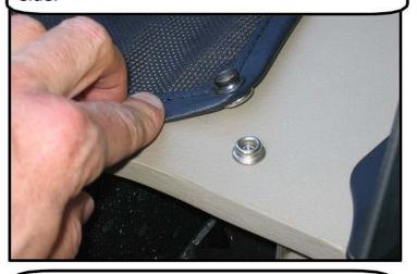
**Step 5 Cont:** Attach the silver snap hooks to the these steel brackets located behind the front seats.
