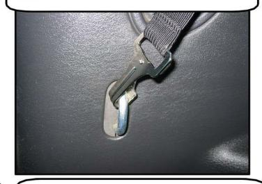
**Step 6 Cont:** These clips will then pull the wind deflector tight. You may need to make a final adjustment of the top straps on the roll bar to smooth out the wrinkles.
