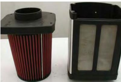
The velocity stack with filter is now out of the power box body.
