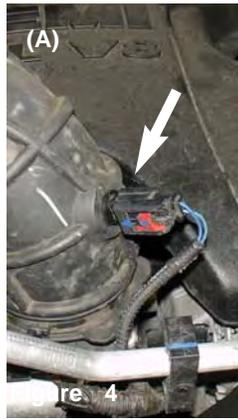
**Figure 4 (A)** Stock air temp sensor on factory air duct.
