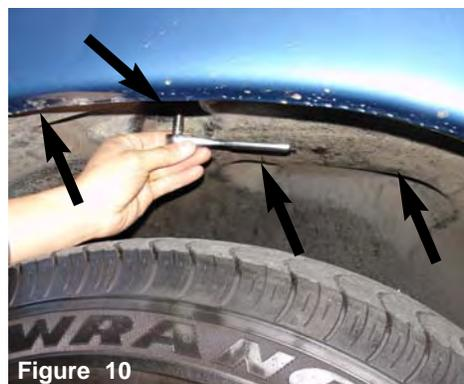
**Figure 10** The six 8mm screws are removed from the plastic wheel well cover as shown above. An additional two screws are under the plastic cover.
