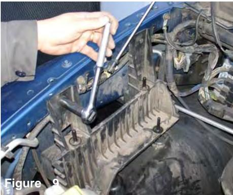
**Figure 9** Use a 13mm socket and ratchet to remove the two bolts holding the air box support bracket to the fender well.
