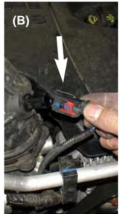
**Figure 4 (B)** Unclip harness from air temp sensor.
