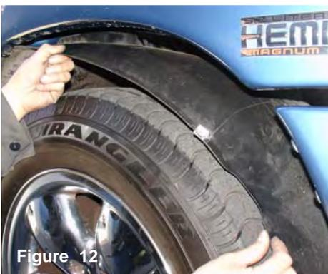
**Figure 12** With all six screws removed from the wheel well cover, peel back on the plastic cover to access the remaining two 8mm bolts.
