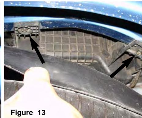
**Figure 13** Use a 13mm socket and ratchet to remove the 2 remaining bolts holding the air box bracket shown in figure 9. Now reinstall the plastic wheel well cover.
