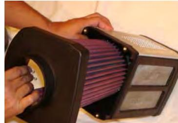
Pull the velocity stack base with the filter that is attached to the velocity stack.
