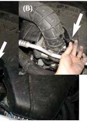
**Figure 5 (B)** Firmly pull air temp sensor out of factory air duct. This sensor will be re-used later.
