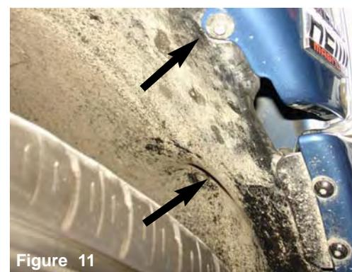
**Figure 11** The two additional 8mm screws are located directly towards the front of the wheel well.
