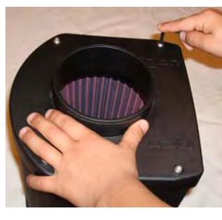
Unbolt the four- m6 x 20mm screws from the velocity stack base located to the center of the base. Now separate the base from the velocity stack.
