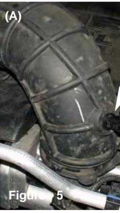
**Figure 5 (A)** Air temp sensor with harness removed.
