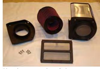
Here is a group shot of the components that goes into the power-box. The filter and screens can now be cleaned with a simple shop-vac.
