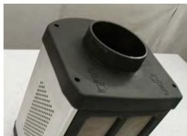
The four m6 x 20 bolts have been removed from the top of the velocity stack,
