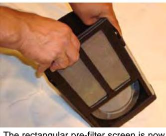
The rectangular pre-filter screen is now slipped out of the channel along the body of the power box.
