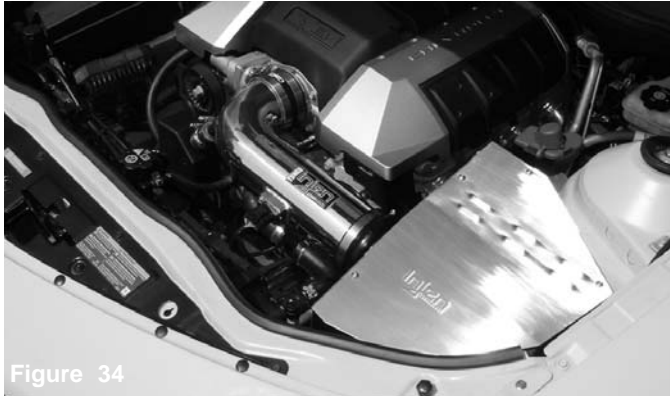
Figure 32 Secure cover using M6 button head screws and tighten using 4mm allen key.
