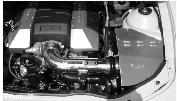
Figure 32 Secure cover using M6 button head screws and tighten using 4mm allen key.
