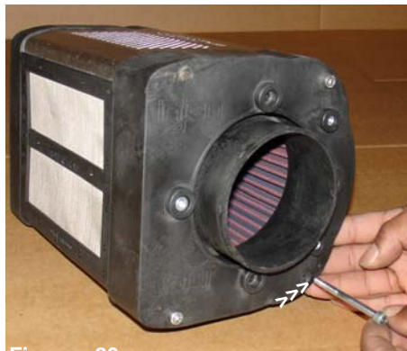
Figure 20 The m6 x 65mm bolt is loosened and removed from the velocity stack base.
