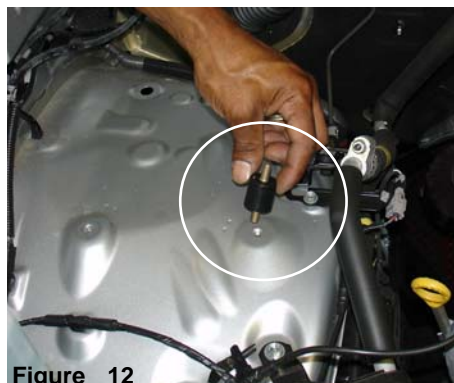
Figure 9 The mass air flow sensor is now lifted from the air box cleaner. The mass air flow sensor will be installed on the intake further on in the instructions.
