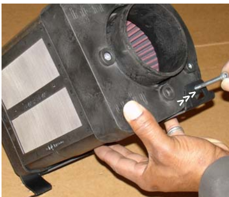
Figure 25 The m6 x 65mm bolt is screwed and fastened to the velocity stack base.
