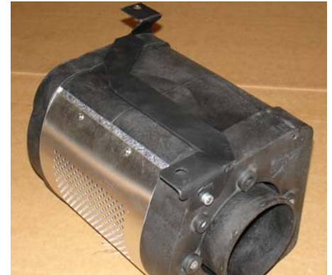
Figure 26 The bolts on both ends are now tightened. View of the power box upside down for better understanding.
