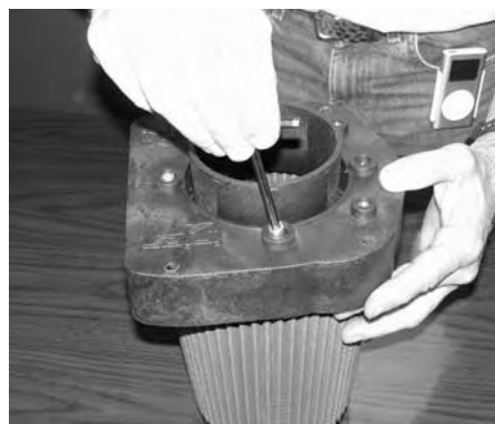
Unbolt the four- 12mm screws from the velocity stack base located to the center of the base. Now separate the base from the velocity stack.
