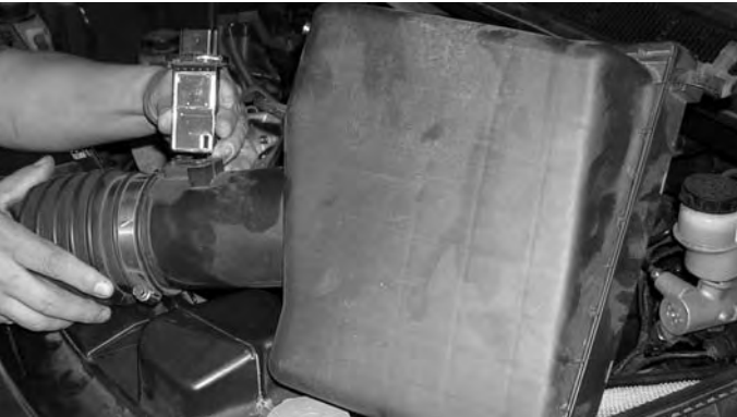
Remove screws holding the sensor in place and carefully slide the mass air sensor out of the sensor pad located on the air box outlet.
