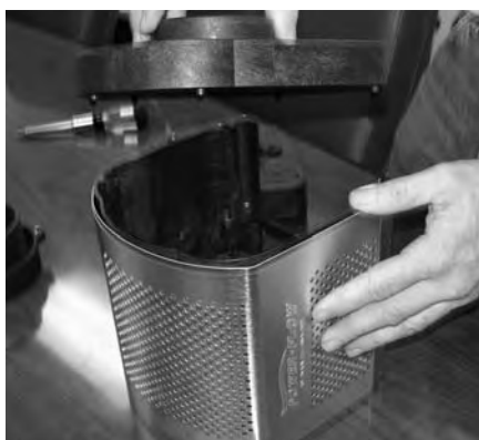
Once the screws have been removed, separate intake air stabilizer from the Power-box body.
