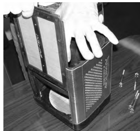
With the velocity stack base out of the way, the rectangular pre-filter screen will now slide out of the Power-box channel.
