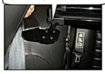
**Step 3 Cont:** It is very important that the bracket sits UNDER the seatbelt strap. As shown in the photo below.
