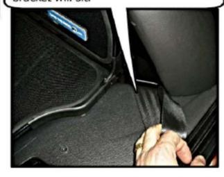
**Step 3:** Lower the front bracket on one side into the hole and release the seatbelt strap. Repeat these steps on the other side.
