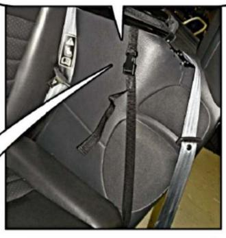
Step 4 Cont: The front silver hooks attach to the bottom of the trim pannel behind the seatbelt retractor on the floor. The other end clips into the strap above, near the front bracket.
