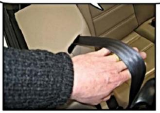
**Step 2 Cont:** Pull the seatbelt strap up to show the hole where the front bracket will sit.
