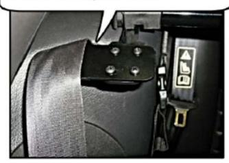
IMPORTANT: NEVER ALLOW THE BRACKET TO SIT ON TOP OF THE SEATBELT AS SHOWN HERE.
