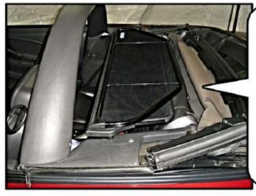
Place the folded wind defector into the back seat area. For the first few times you install the wind deflector, it is easier to have someone help hold the wind deflector at the other end while you adjust the seat belt straps over the brackets.
