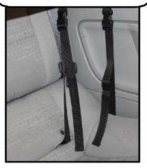
On your rear seats there will be a small circle with a child seat picture to show you where the anchors are. The black snap hooks are inserted with the snap facing down. Slide the hook into the hole, press down and then pull back up towards you to secure it into place.
