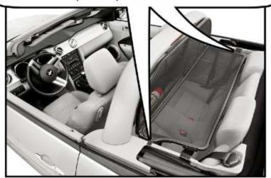
The wind deflector stays securely in place using four straps which attach to your cars child seat anchoring system and the side trim panels.
