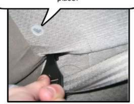
The two front straps will clip onto a hole on the bottom of the side trim panel, below the rear speakers.
