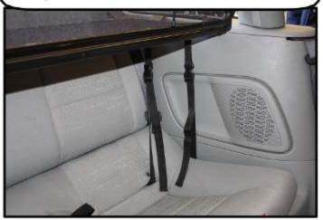
Step 1: Start by lowering the folded wind deflector into the back seat area so the brackets fit onto each side of the trim panel.
