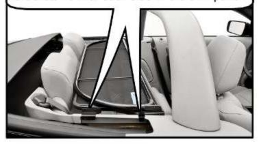
Below is a close up to show the two brackets on the trim panel on one side. You may need to adjust the rear brackets to fit tightly against the trim panel
