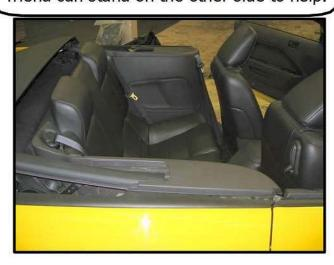
**Step 3 Cont:** The front brackets fit into the space behind the hole where the seat belt comes out of. The brackets are designed not to interfere with the seat belt.
