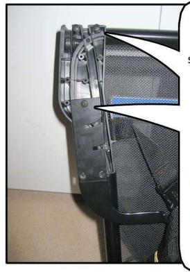
step 1: When your wind deflector was shipped to you the front brackets had to be lowered to fit into the box. You need to remove the top two screws using a #2 philips (This is a very common screw driver and the end of the screw looks like an X) Do not remove the bottom screw.
