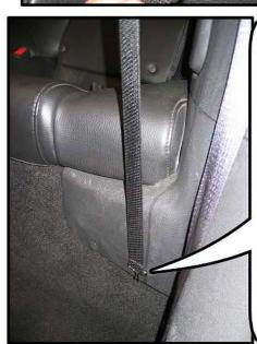
Step 6: The front silver hook straps attach to the bottom of the trim panel below the back seats. Attach the silver hooks on both sides.
