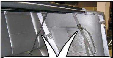
**Step 6 Cont:** Next attach the four straps. The two black snap hook straps attach near the back brackets and the two silver hook straps attach to the buckle under the front brackets.
