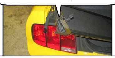
**PLEASE NOTE:** If you try to put the wind deflector in your trunk with the front brackets facing the wrong way (frontwards) it will not fit properly. If you do manage to get it in, it will be very difficult to remove.
