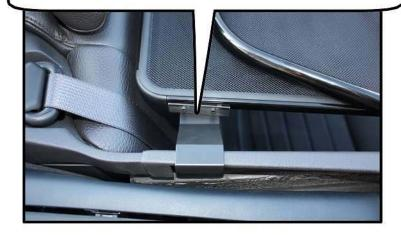
**Step 4 Cont:** The rear brackets may need to be adjusted so they fit tight against the trim panel. The adjustment is made by adjusting the two screws underneath the wind defelctor.
