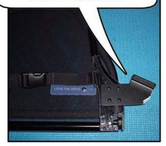
**Step 2:** You are now ready to install your wind deflector. With the top down, start by placing your hand underneath the front seatbelt strap.
