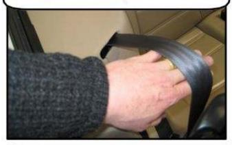
**Step 3:** Lower then front bracket on one side into the hole and release the seatbelt strap. Repeat these steps on the other side.
