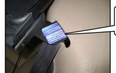
IMPORTANT: NEVER ALLOW THE BRACKET TO SIT ON TOP OF THE SEATBELT AS SHOWN HERE.
