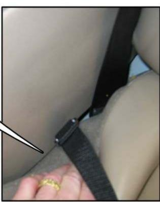
Step 4 Cont: The black snap hook straps then clip into the strap attached at the rear bracket. PLEASE NOTE: If you have a Mustang that was built after 2002 you will have a child safey anchoring system which you can use to lock the black snap hooks into instead. Notice the small baby seat logos above where the anchors are located.
