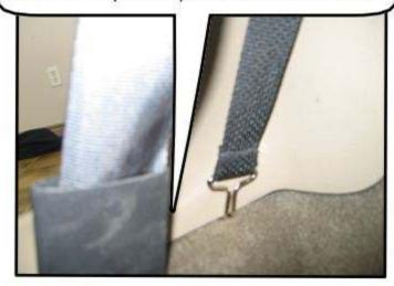
**Step 4 Cont:** The rear black snap hooks attach to the bottom of the trim panel beside the backseat. There is a small square cut out for the hook. Insert the black snap hook here.
