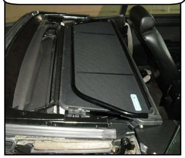
The front brackets will sit on top of the trim panels, as shown in the photo below.
