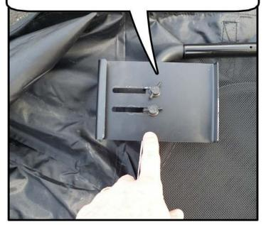
Lay the wind deflector in rear seat area. The front and rear brackets will rest on the rear trim panel.
