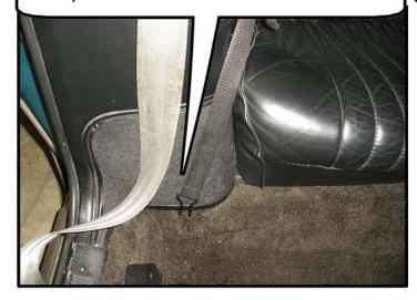
Pull the straps down to tighten on both sides.
