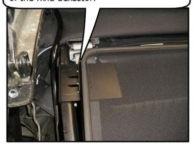
The straps attach to the bottom of the trim panel.
