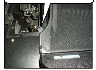
Slide the rear brackets back so that they lock into the trim panel. Tighten the thumb screws on both sides, from the under side of the wind deflector.
