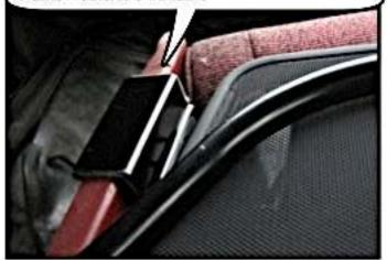
STEP 5: THERE ARE TWO STRAPS THAT ATTACH TO THE BOTTOM OF THE TRIM PANELS. THE BLACK HOOK WILL ATTACH TO THE BOTTOM OF THE TRIM PANEL
