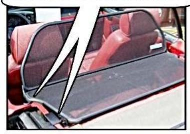
STEP 1: THE REAR BRACKETS ARE ADJUSTABLE. START BUT LOSSENING THE THUMB SCREW. PUSH THE BRACKET SO IT IS 3/4 EXTENDED
