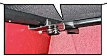
THE STRAPS WILL ATTACH TO THE BUCKELES ON THE BOTTOM OF THE WIND DEFLECTOR.
