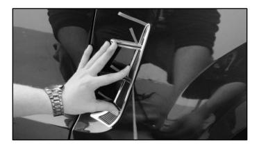
**4.)** Continue holding the Quarter Molding and pull the front tab toward the bottom of the vehicle as shown below. The front tab must be pulled behind the three protrusions. Apply light pressure to the insert where the lining has been removed.
