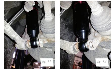
4. Align and attach the lower shock mount with the control arm (Fig. 11). Torque to 71 Nm (52 lb.-ft.). (Fig.12)
