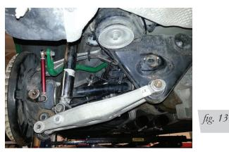
4. Remove the cam bolt from the inner control arm pivot point and remove the control arm (fig. 14).
