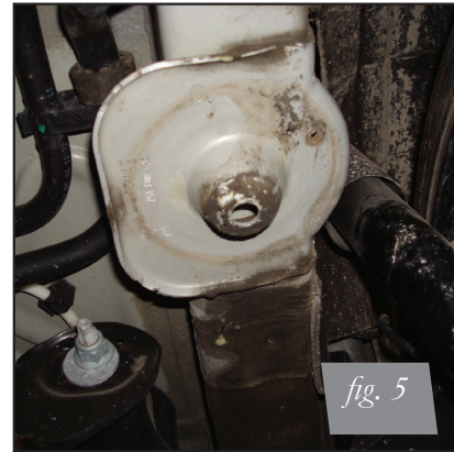
Previously Cut Spring Perch with Aftermarket Shock
