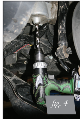
Previously Cut Spring Perch with Aftermarket Shock
