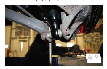
4. Spin the red locking collar against the lower eye mount. Tighten collar 1/4 turn beyond hand tight (Fig. 19).
