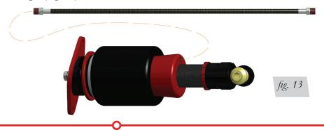
2. Remove the flexible adjuster knob and route flexible adjuster extension through the previously drilled hole. Attach the upper mount bracket to the chassis with the previously removed bolts (Figs. 14-16). Torque to 56 Nm (41 lb.-ft.).
