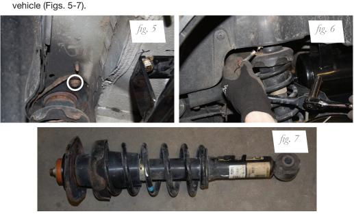
3. Remove the two upper mount bolts and remove the shock assembly from the
