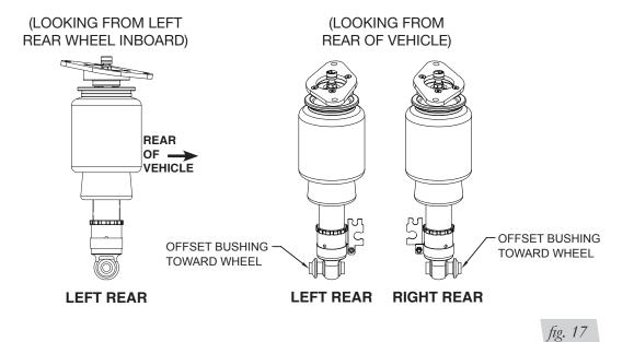
3. Align the lower eye mount with the offset bushing against the mounting surface. Install the lower bolt but do not torque at this time (Torque the lower mount bolt when the vehicle is at ride height.) (Fig. 18).
