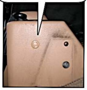
STEP 1 CONT: TO REMOVE THE PUSH PIN USE A THIN SCREW DRIVER AND GENTLE LIFT THE MIDDLE SECTION OF THE PUSH PIN
