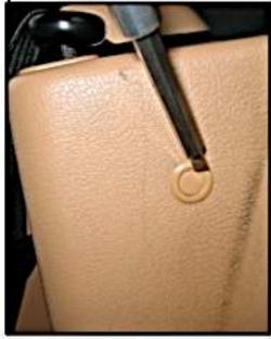
STEP 1 CONT: ONCE THE MIDDLE HAS BEEN PUSHED OUT YOU CAN REMOVE THE PUSH PIN. DO THIS ON BOTH SIDES
