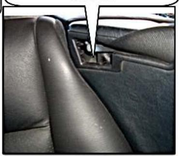
STAND BESIDE THE REAR SEAT ON THE OUTSIDE OF THE CAR. START BY INSERTING THE REAR BRACKET IN THE SPACE BELOW THE SEAT BELT ON THE OPPOSITE SIDE TO WHICH YOU ARE STANDING. THEN INSERT THE REAR BRACKET ON THE SIDE CLOSEST TO YOU
