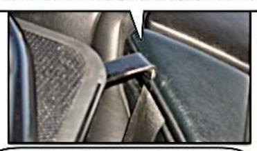
THEN SET THE FRONT OF THE WIND DEFLECTOR DOWN AND THE FRONT BRACKETS WILL REST ON THE SIDE TRIM PANEL
