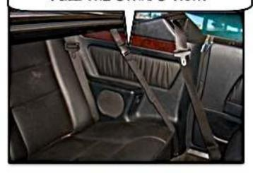
THE TWO BRACKETS SHOULD SIT FLAT ON THE TRIM PANEL AND SHOULD NOT INTERFERE WITH THE REAR SEAT BELT
