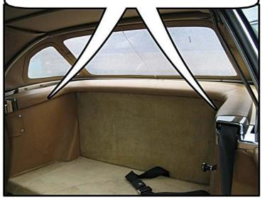
**Step 1:** Start by placing the wind deflector into the area behind the front seats, on top of the lid. Make sure that it is sitting straight.
