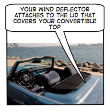
THE MB 113 WIND DEFLECTOR ATTACHES WITH THE TWO BRACKETS IN THE REAR AND TWO LATCHES IN THE FRONT
