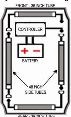
Organize the tubes outside the perimeter of the vehicle then test functionality before moving forward with your installation.
