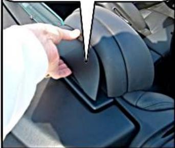
NEXT PLACE THE WIND DEFLECTOR SO IT SITS ON THE REAR HEAD RESTS. MAKE SURE THAT THE BLACK SNAP HOOKS ARE BEHIND THE REAR SEAT HEAD RESTS
