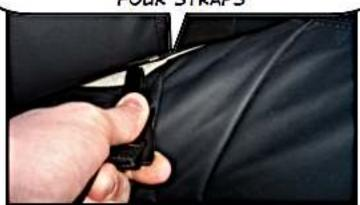
NEXT ATTACH THE FOUR BLACK SNAP HOOKS TO THE FOUR BUCKLES ON THE WIND DEFLECTOR
