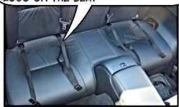
THE BLACK SNAP HOOKS ARE INSERTED WITH THE SNAP HOOK FACING DOWN
