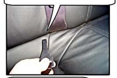
WITH ONE HAND PUSH DOWN ON THE BOTTOM OF THE REAR SEAT AND SLIDE THE SNAP HOOK IN AND THEN PULL BACK TO ATTACH IT TO THE ANCHOR SYSTEM. DO THIS FOR ALL FOUR STRAPS
