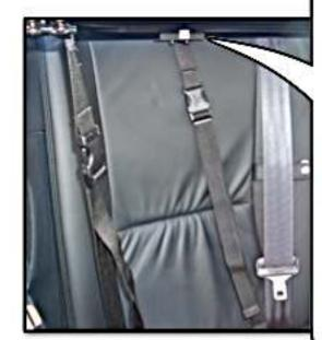
THE TWO STRAPS IN THE CENTER OF THE BACK SEAT ATTACH TO THE **FEMALE** BUCKLE AT THE BACK OF THE WIND DEFLECTOR. THE TWO OUTSIDE STRAPS ATTACH TO THE BUCKLES ON THE SIDE OF THE WIND DEFLECTOR
