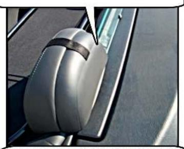
NEXT WE ARE GOING TO ATTACH THE FOUR BLACK SNAP HOOKS TO THE CHILD ANCHOR SYSTEM IN THE REAR SEAT. THE ANCHORS ARE LOCATED BETWEEN THE TOP AND BOTTOM PART OF THE SEAT. LOOK FOR THE LOGO ON THE SEAT
