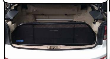
To store the wind deflector, turn handle of the front barrel bolts to the front of the wind deflctor and slide back. Then turn the handle down to lock it. Loosen the thumbscrews (towards passenger side) and close the rear brackets flat.
