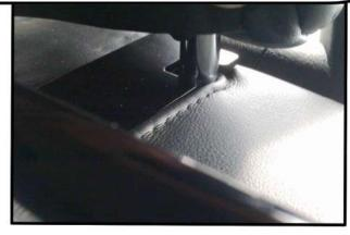
Once both the rear brackets are locked into place, reach under and tighten the thumbscrews on both of the rear brackets. Turn towards the drivers side.
