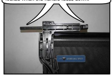
The rear brackets are then turned to 90 degrees so they will lock into place with the rear seat head rests. See next photo.
