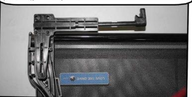
The barrel bolt should be put in first with the rear brackets facing up. The wind deflector should always be stored in its storage bag.
