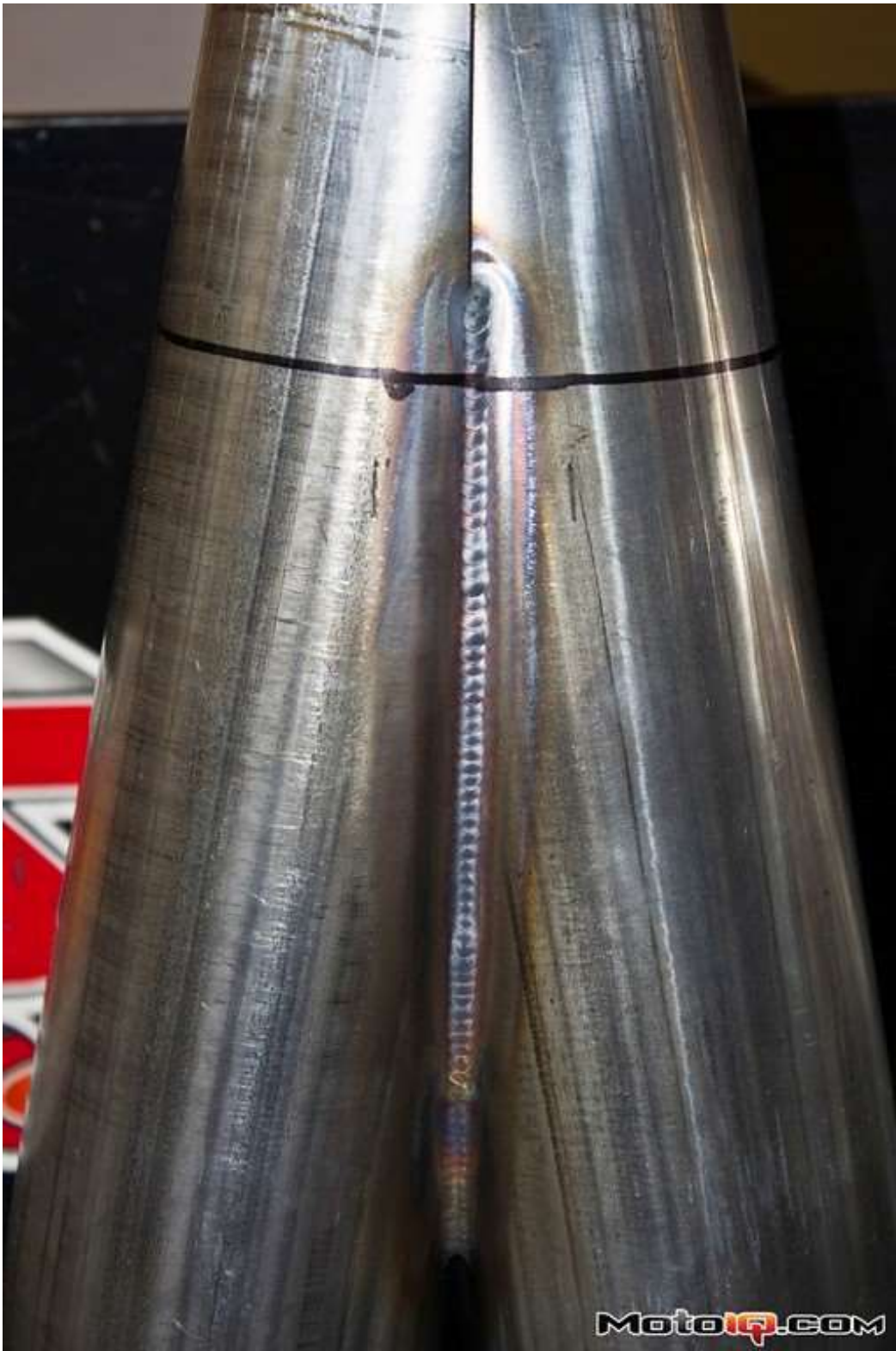
Here we can see the beautiful TIG welds performed on a merge collector by the craftsmen at Kooks.
