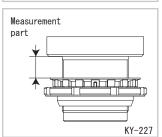
1. After installing the shock absorber on the vehicle, measure the area marked in the Figure, and adjust to match the reference values shown below.
