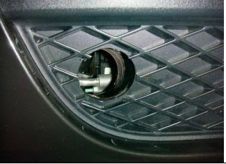
5 Using silver 10mm bolt on lower flange of drivers side headlight attach Fresh Air mounting bracket:
