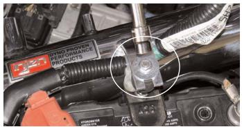
Place the m6 flange nut and fender washer over the intake bracket and vibramount stud. Take the m8 socket and rachet and semi-tighten the flange nut for
