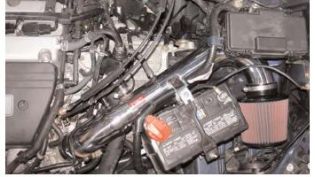
Congratrulations! You have just completed the installation of this intake system. Periodically, check the fitment of the intake system in order to prevent damage to the intake system and/or engine components.
