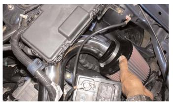
Press the filter neck over the end of the intake system until it butts up against the velocity stack.
