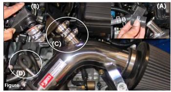
Press the 1 1/8" x 2" hose over the large port on the intake, use the two mini clamps in this kit to secure the hose(A). Press the assembled vent chamber port into the large hose on the intake(B). This illustration shows a filter on the end of the intake to be used as a short ram.
