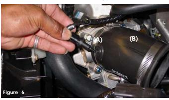
Press the sensor grommet in this kit into the hole in the elbow. Place the clamps over the beaded elbow and press the assembled elbow over the throttle body(B). Position the elbow in the correct direction and press the air temperature sensor into the sensor grommet (A).
