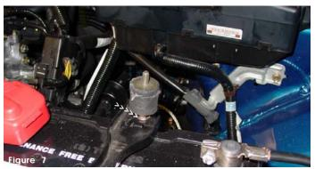
Take the male/female vibra-mount and screw it over the threaded battery post. Do not bottom out the vibra-mount a full 20 turns will be more than enough.
