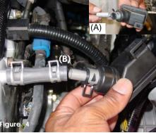
Press the 1 1/2" x 1/2" aluminum coupler into the vent chamber (A) and connect to breather line(B). Press the coupler into the chamber then into the stock breather hose on the crankcase(B).
