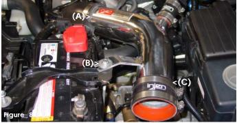
Press the primary intake into the elbow on the throttle body(A) and line up the bracket on the intake to the vibra-mount stud(B), use the m6 nut and washer to hold the intake in place. The 3" hose on the end of the intake is only used on the RD1680 for the secondary intake (C).
