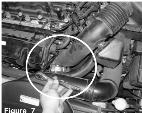
Figure 7 Use a 10mm socket and ratchet to loosen the clamp on the air duct connected to the throttle body
