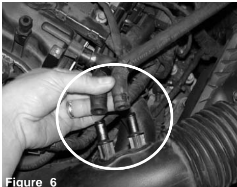
Figure 6 Both breather lines removed from air duct
