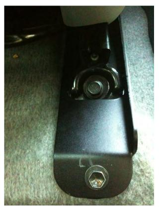
Step 9- In the front area; lay your factory seat on top of the EMS brackets and line up seat front holes with EMS front holes. Finger tighten front 2 feet with provided black EMS bolts.
