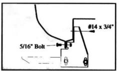
5. Drill 5/16"" diameter hole through pinch weld at marks. Bolt FL39 flat bracket to pinch weld with 5/16" x 3/4" bolt and nut, then use #14 x 3/4" self-drilling screw in top hole into rocker panel.
