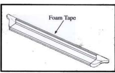
Apply foam tape strips to GlaStep edge.
