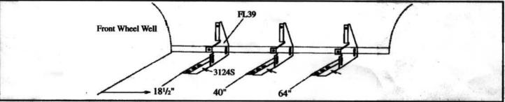
3. Measure from front wheel well, back 18<sup>1</sup>/<sub>2</sub>", 40" and 64". Mark these bracket location centers. Note: Steel plates have been inserted under fiberglass to mount brackets securely using self-drilling screws.
