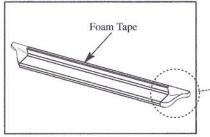
6. Apply foam tape to top edge of GlaStep. Remove protective strip from top edge of foam tape.
