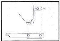
5. Drill 5/16" diameter holes in pinch weld at marks. Bolt brackets FL43 to pinch weld using 5/16" bolts and nuts, then secure to inner rocker panel using #14 x 3/4" self-drilling screws through AS01.
