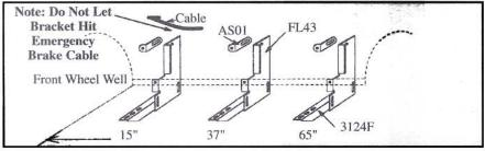
3. Measure from front wheel well, back 15", 37" and 65". Mark these bracket locations. Note: Steel plates have been inserted under fiberglass to mount brackets securely using self-drilling screws. Double check your marks to be sure they line up with the steel plates before drilling.
