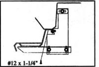
7. Secure GlaStep to body with #12 x 1-1/4" self-drilling screws with rubber washers.
