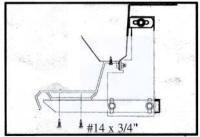
8. Position step on brackets and tight to truck body. Screw step to bracket using two #14 x 3/4" self-drilling screws per bracket and adjust GlaStep to body. Tighten all bolts to 18 foot pounds.
