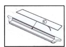
9. Place pad on step. Peel off tape backing to secure. Don't forget the Owens label!
