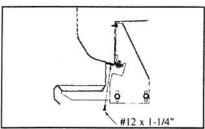
Secure GlaStep to body with #12 x 1-1/4" self-drilling screws with rubber washers.
