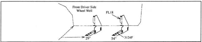
Measure from front wheel well, back 29" and 54". Mark these bracket location centers. Note: Steel plates have been inserted under fiberglass to mount brackets securely using self-drilling screws.
