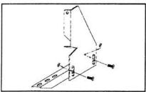
Assemble FL18 to 3124F using two 5/16" nuts and bolts. Do not tighten at this time.
