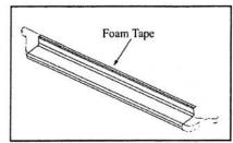
Apply foam tape strips to GlaStep edge.
