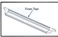
Apply foam tape strips to GlaStep edge.
