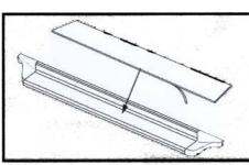
9. Place step pad on GlaStep. Peel off tape backing to secure. Don't forget the Owens label!
