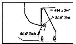
5. Drill 5/16"" diameter hole through pinch weld at marks. Bolt FL18 flat bracket to pinch weld with 5/16" x 3/4" bolt and nut, then use #14 x 3/4" self-drilling screw in top hole into rocker panel.
