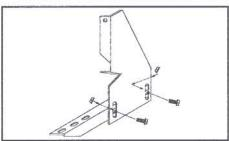
4. Assemble FL18 to 3124F using two 5/16" nuts and bolts. Do not tighten at this time.
