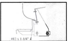
Secure GlaStep to body with #12 x 1-1/4" self-drilling screws with rubber washers.
