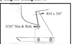
5. Drill 5/16"" diameter hole through pinch weld at marks. Bolt FL15 flat bracket to pinch weld seam with 5/16" x 3/4" bolt and nut, then use #14 x 3/4" self-drilling screw in top hole into rocker panel.
