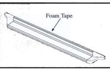
Apply foam tape strips to GlaStep edge.
