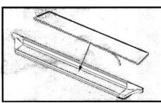
9. Place step pad on GlaStep. Peel off tape backing to secure. Don't forget the Owens label!
