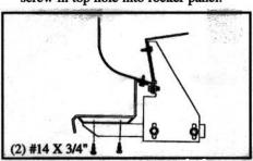
Secure step support bracket to bottom of GlaStep using two #14 x 3/4" selfdrilling screws per bracket. Tighten all bolts to 18 foot pounds.
