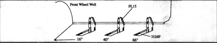
3. Measure from front wheel well, back 16", 40" and 66". Mark these bracket location centers. Note: Steel plates have been inserted under fiberglass to mount brackets securely using self-drilling screws.
