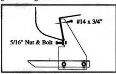
5. Drill 5/16"" diameter hole through pinch weld at marks. Bolt FL15 flat bracket to pinch weld seam with 5/16" x 3/4" bolt and nut, then use #14 x 3/4" self-drilling
