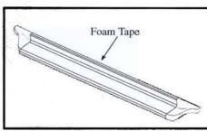
Apply foam tape strips to GlaStep edge.
