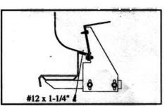
Secure GlaStep to body with #12 x 1-1/4" self-drilling screws with rubber
