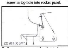
8. Secure step support bracket to bottom of GlaStep using two #14 x 3/4" self-drilling screws per bracket. Tighten all bolts to 18 foot pounds.
