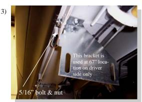
Attach FL229 bracket at 67" location on driver side only with 5/16" bolt and nut and one 3/4" long self drilling screw. Pre drill hole for self taping screw with 1/8" drill bit.
