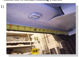
Measuring from the front wheel well, measure towards the rear of the vehicle. At locations 19" (20" on Pass. Side), 32",50" and 67" make a mark on the pinch weld, this is where the brackets will be attached.
