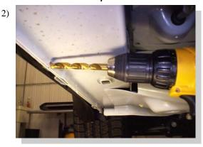
At each mark drill a 23/64" hole through the pinch weld.
