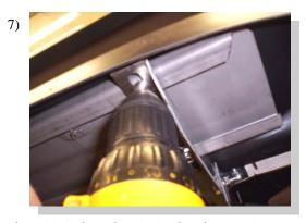
Place 67085 board on 3124F brackets, position board so it fits snug up against the vehicle and is level. Attach with 3/4" long self drilling screws. Tighten bolts holding the 3124F 's to the flat brackets.
