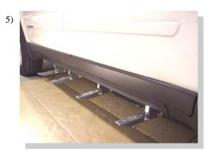
Attach one 3124F to each bracket using 5/16" bolts and nuts. Do not tighten.
