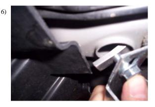
Insert 5/16" flanged bolt through CB65 into retaining nut, then insert retaining nut into the forward hole in the frame for the front bracket to mount to.
