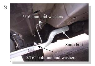
Attach CB64 and "Z" bracket to vehicle as shown at the rear location.
