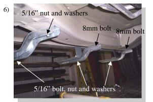
Attach CB64 to 36" 58" location and CB65 to 17-1/2" as shown. Tighten all hardware.
