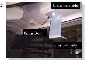
Attach the front two "Z" brackets to factory holes with 8mm bolts. The rear "Z" bracket will attach with supplied bolt/wire and nut . The under bent side of Z bracket goes against body.
