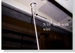
Remove the reward rubber plug and insert the bolt with a wire through the hole as shown. "Fish" the wire towards the rear of the vehicle and insert the bolt through the rear hole.
