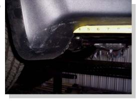
Brackets will be attached using factory mounting locations at 17 1/2", 36" and 58".
