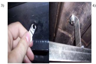
Insert 8mm pull nut into holes in rocker panel where you removed rubber plug. Insert 8mm bolt with washer through BT69 and into 8mm pull nut at 10" 34" location. At 64.5" insert 8mm bolt with washer through slot in FL224D/P into 8mm pull nut. Snug but don't tighten.
