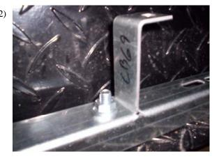
Attach BT69 to channel brackets with 5/16" flanged nut and bolts.
