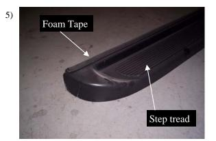
Apply foam tape and step tread as shown in picture. Center step tread between the ends of the board and keep close to outside edge.
