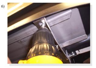
Position board between wheel wells for best fit. Install self taping bolts through bracket into the shoulder of the steel channel on the bottom of the board. Don't attach lip of board directly to vehicle.
