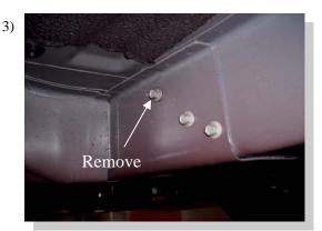
On the drivers side at the 11 1/2" location remove the upper bolt shown on the vehicle frame. Do not discard.
