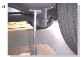
Remove the small stone protector that is in front of the rear wheel. This will not be reused.
