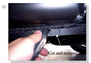
Measure from front wheel well back and make a mark at 11 1/2" (13" on passenger side), 26", 43" and 59". At each mark, remove about a 1-1/4" wide piece of the cladding covering the pinch weld.
