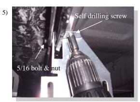
Attach an FL123 to the 26" location using one 5/16" bolt and nut through the pinch weld and one 3/4" long self drilling screw.
