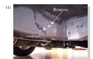
On the passenger side at the 13" location remove the upper bolt shown on the vehicle frame. Do not discard.
