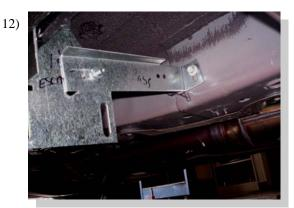
Assemble FL123 to BT55 as shown. Using a 5/16" bolt and nut attach bracket to the pinch weld and the BT55 to the body using the bolt removed in step 5.
