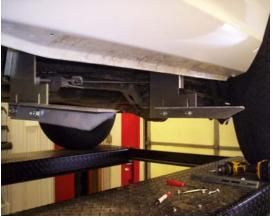
Attach a 3124F angle bracket to the FL221 and FL222D & P with 5/16" bolts and nuts. Snug but do not tighten at this time.
