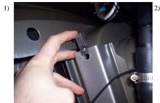
Locate the front bed cross member and install clip nut as shown in **Fig. 1.** If no hole is present you will have to drill a 1/2" hole and insert 8mm pull nut as shown in **Fig. 4**
