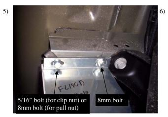
Install FL222D & P using 5/16" flanged bolt (for clip nut only) and 8mm bolt and washers, as in **Fig. 5.**
