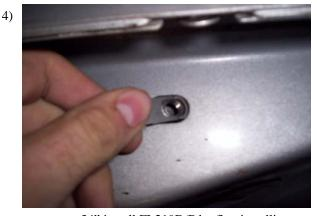
At measurement 34" install FL219D/P by first installing a pull nut into oblong hole in underbody, then insert 1/4" carriage bolt through hole in pinch weld and through bracket, and attach with 1/4" flanged nut. Insert 8mm bolt through bracket into pull nut. Install self tapping bolt through top of bracket into under body. Tighten all nuts and bolts.
