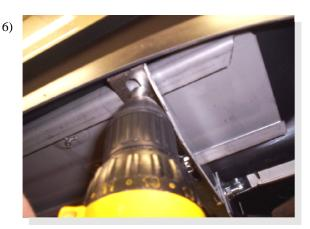
Position board between wheel wells for best fit. Install self taping bolts through bracket into the shoulder of the steel channel on the bottom of the board.
