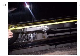
Measure from front wheel well towards the rear and make a mark on pinch weld at 16" 34" and 64". There should be a hole at these locations.
