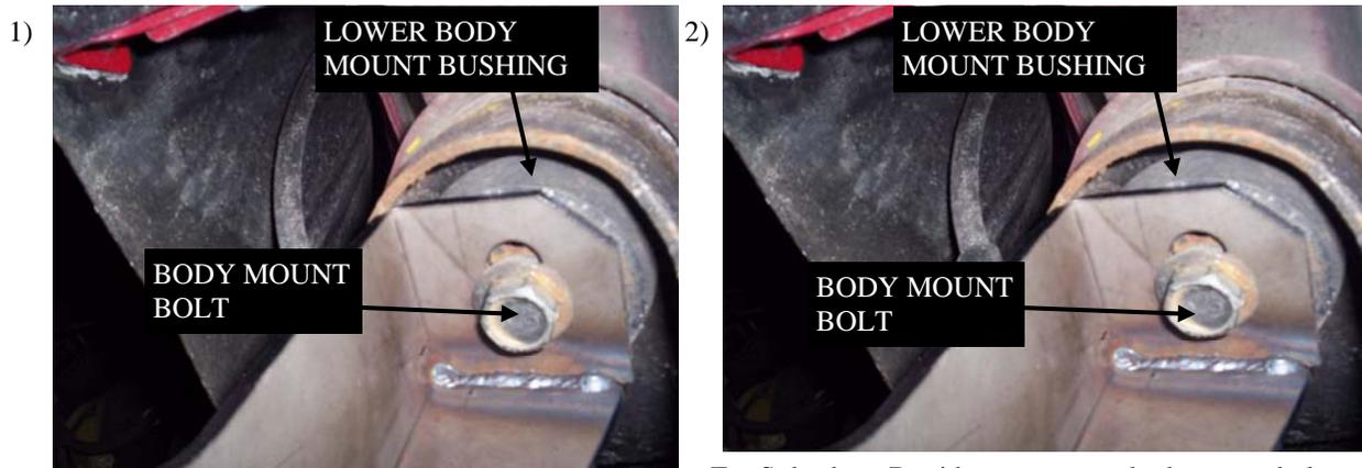
1) Starting at DR side front body mount. Remove body mount bolt, place FL215 between the bolt and the lower body mount bushing, retighten body mount bolt. Repeat steps for pass side using FL207
