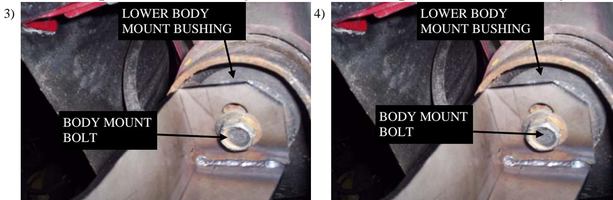
3) At Dr side rear body mount. Remove body mount bolt, place FL213 between the bolt and the lower body mount bushing, retighten body mount bolt. Repeat steps for pass side using FL209
