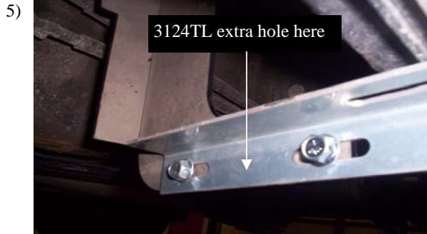
Std cab: Attach 3124TR at Dr rear and pass front location, ( **NOTE, 3124TL will have extra hole where indicated above.**) attach 3124TL at Dr front and pass rear location using 5/16" flanged nut and bolts as shown.
