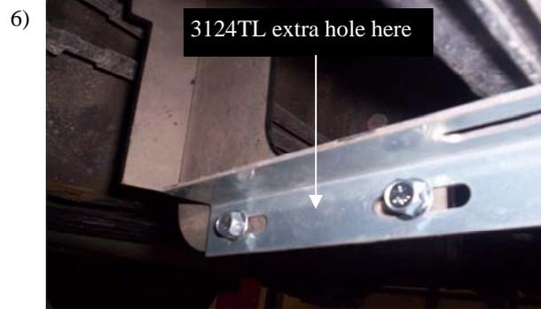
Ext/Crew cab: Attach 3124TR at Dr rear/middle, pass front/middle location, ( **NOTE, 3124TL will have extra hole where indicated above.**) attach 3124TL at Dr front and pass rear location using 5/16" flanged nut and bolts as shown.
